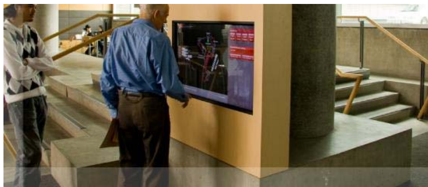
*Touch Screen LCDs were integrated by Horizon Display using optical technology and NEC M46 commercial grade monitors.
